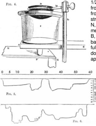
1/2 inches, being 5 1/2 inches from the bottom of 1, and 2 inches from its circumference. Shaking or striking the arm, M, or the vessel, N, produces no appreciable mechanical effect on the board, A B, capable of affecting the balance. Dipping the hand to the fullest extent into the water in N, does not produce the least appreciable action on the balance.
